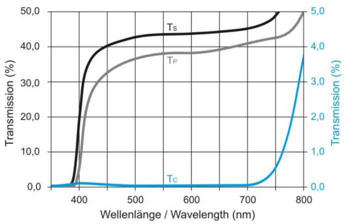
Transmission curve polarisation filter
