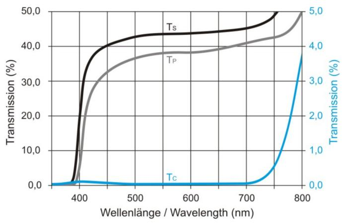
Transmission curve polarisation filter
