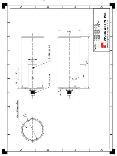
Image 5: Technical Drawings (dimensions in mm)
