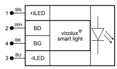
Image 8: Connection diagram vicolux smart light
