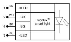
Image 9: Connection diagram vicolux smart light
