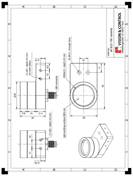
Image 3: Technical drawings (dimensions in mm)
